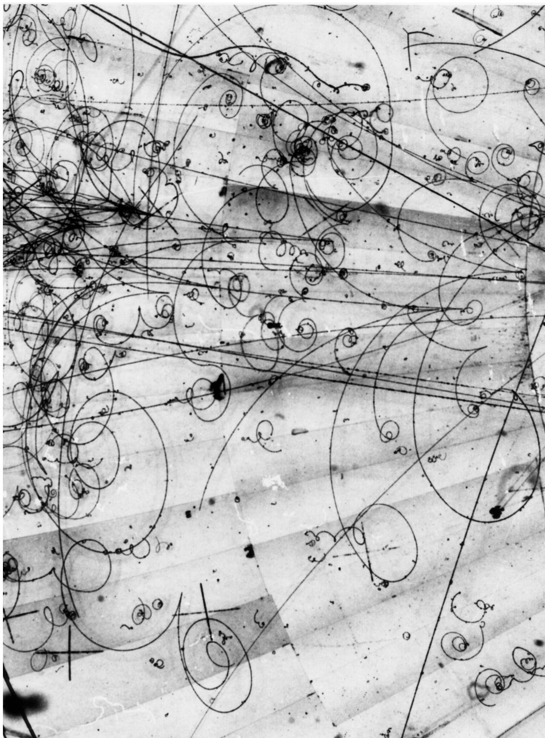
**Figure 1.** Part of a bubble chamber picture. The dark lines are trails of tiny bubbles created as charged particles force their way through a tank of transparent liquid enclosed in a powerful magnet. At P, the main point of interest, a positron (antielectron) in flight meets an electron and annihilation takes place. One of the photons from the annihilation materializes at Q. At E, a different positron seems to change
