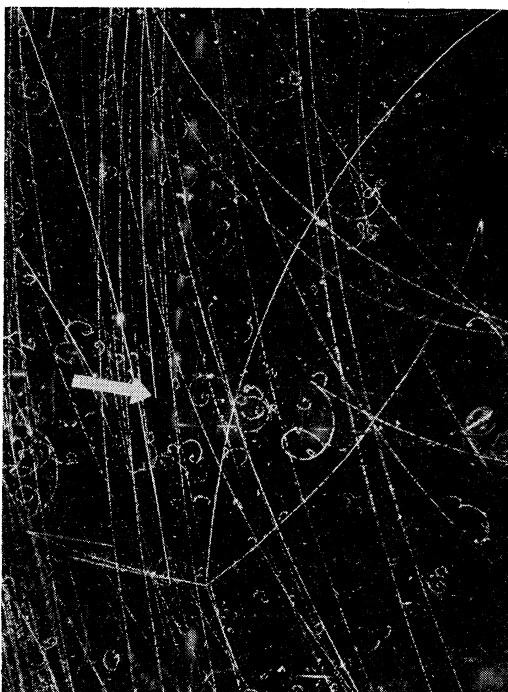
FIG. 3. An antiproton charge exchange. The antiproton is incident from the top and to the left of center, and the antiproton ending is indicated by an arrow. The antineutron from the charge-exchange process annihilates in the lower center of the picture. Five pions are produced in the annihilation with an energy release >1500 Mev.
